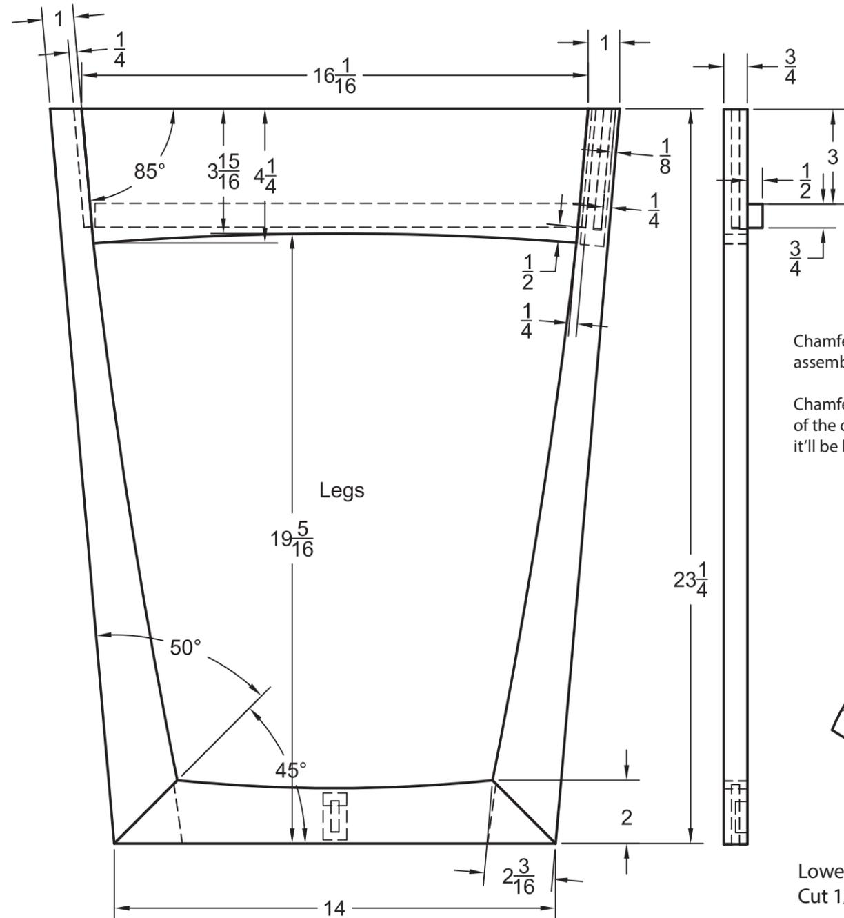
Chamfer all but the top edges of the leg assembly after gluing and sanding.
